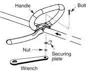
Install the bolt, securing plate and nut as shown in the illustration.
